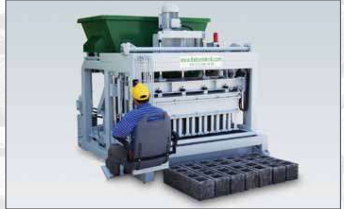
BPM14 - BLOCK MACHINE (12000 piece/day)
