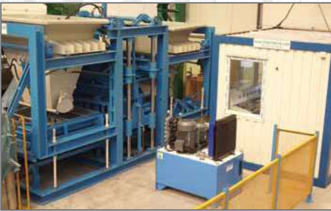
BPM36 - BLOCK MACHINE (1000 m²/day)
