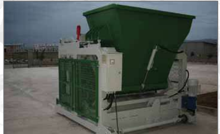
BPM14 - BLOCK MACHINE (12000 piece/day)
