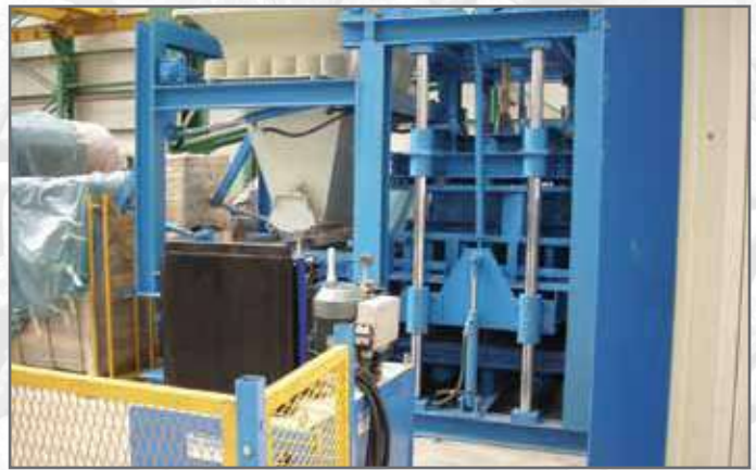
BPM36 - BLOCK MACHINE (1000 m²/day)
